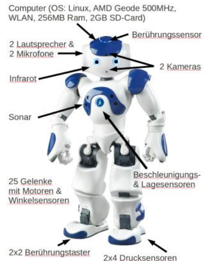
Sensoren des Roboters NAO (© Austrian Kangaroos 2010)
